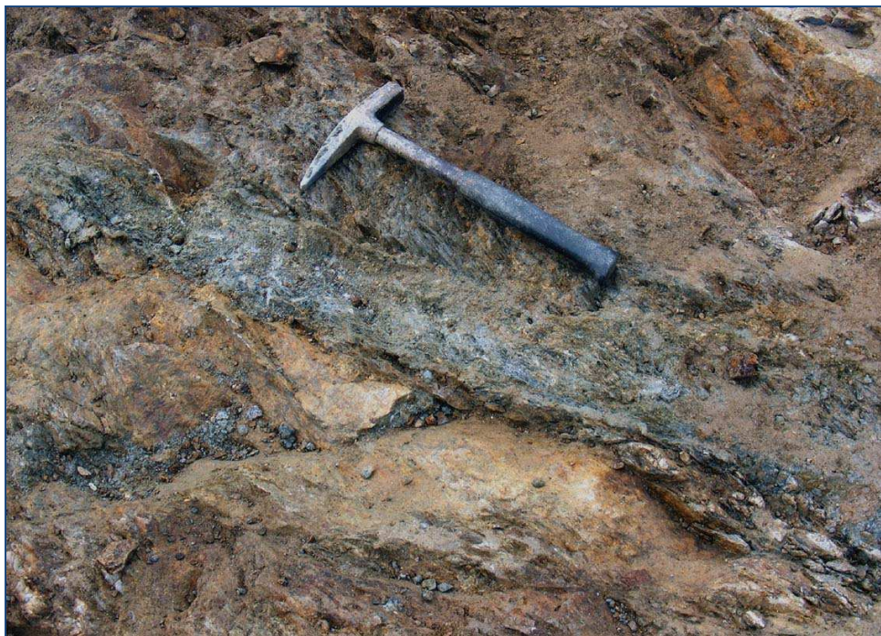
Fig. 45 View of an approx. 5 cm thick filling of a tectonic dislocation in the spent fuel repository (SFR) foundation base in Temelín NPP. The filling consisted of green crumbly clay with shreds of surrounding rocks. The disturbance with the filling was approximately 10 m long and onwards thinned out. Photo by I. Prachař, 2009.
