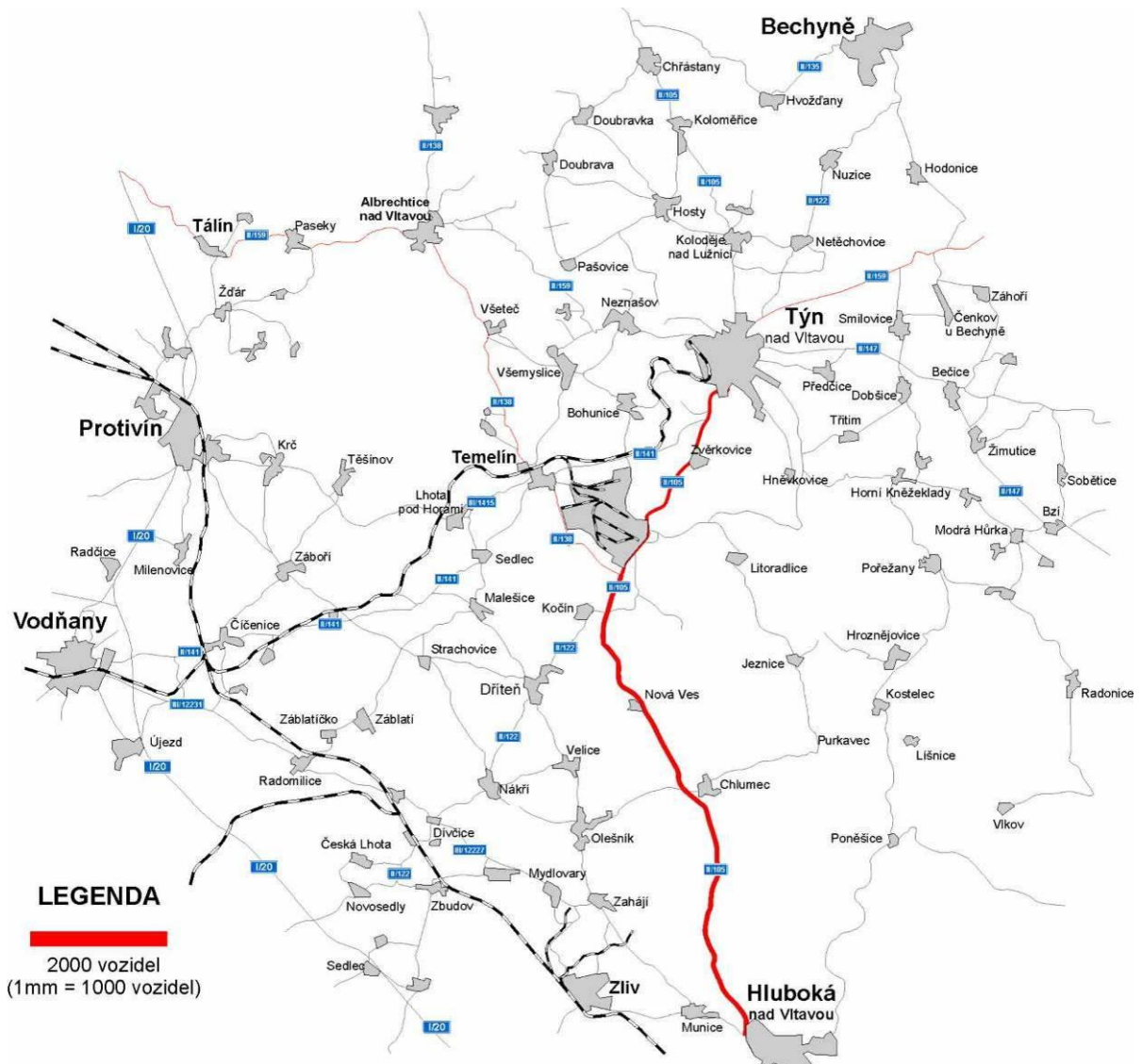
Figure B.II.4: Traffic volumes on roads around NPP Temelín due to NNPP operation
