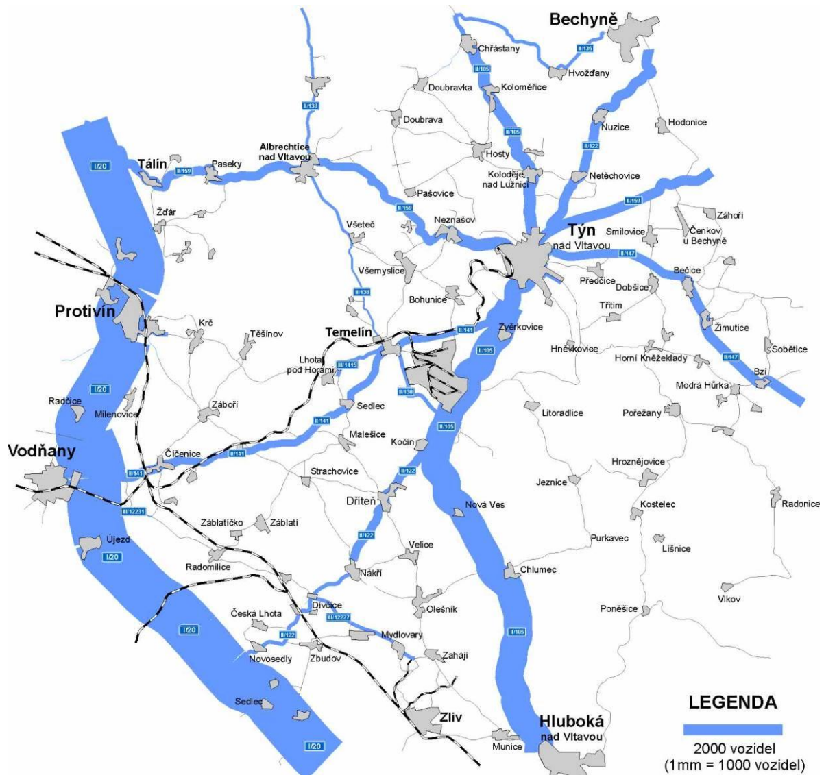
Figure C.2.94: Cartogram of the traffic load of the road network in the broader affected area
